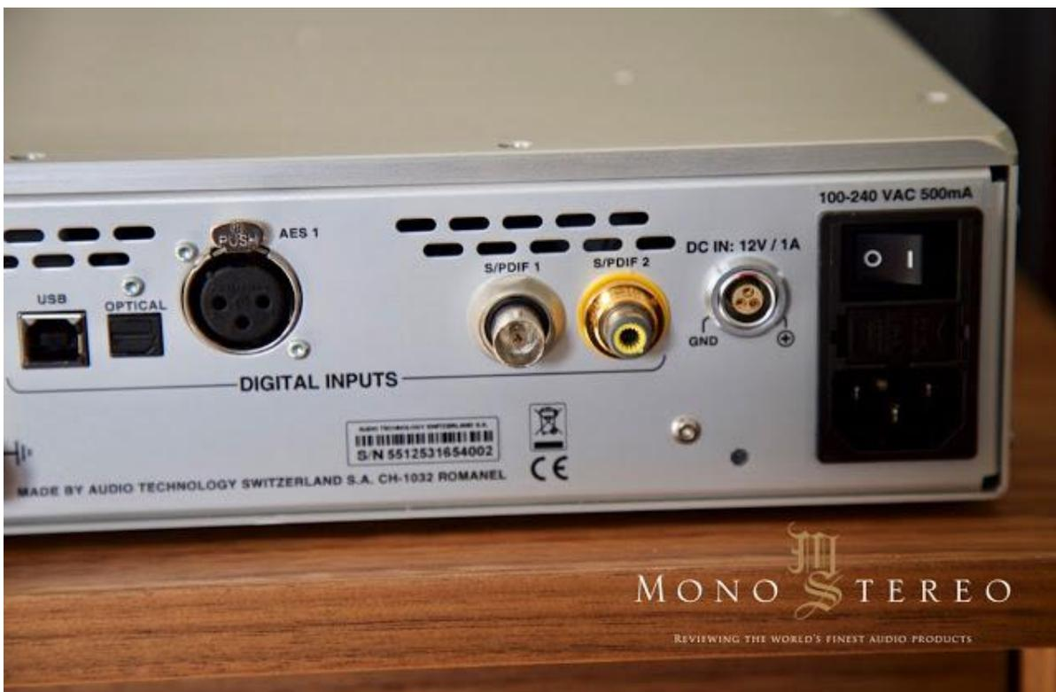
What about the USB input, that's mostly used? Dedicated high speed USB input was developed around the bit perfect circuit, specially programmed for Nagra by the Italian firm Amanero Technologies.
